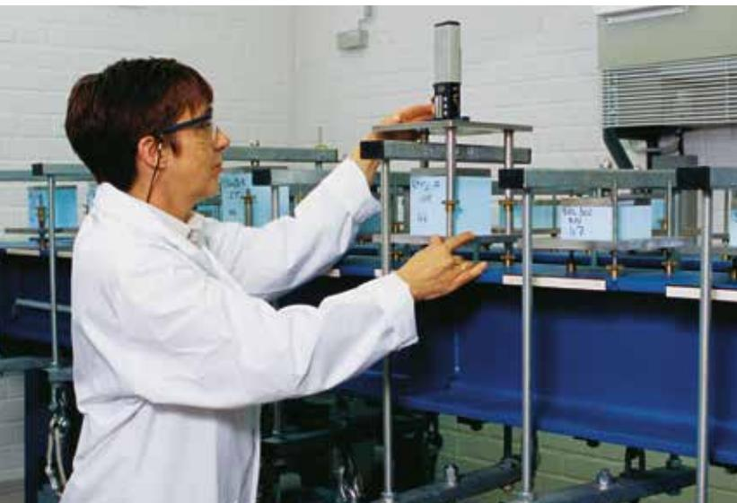
*Fig. 17: Dynamic testing of composite test pieces with STYROFOAM™ core layer material*
