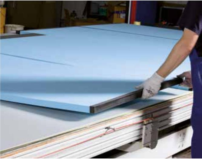
Fig. 10: Aligning STYROFOAM™ panels
