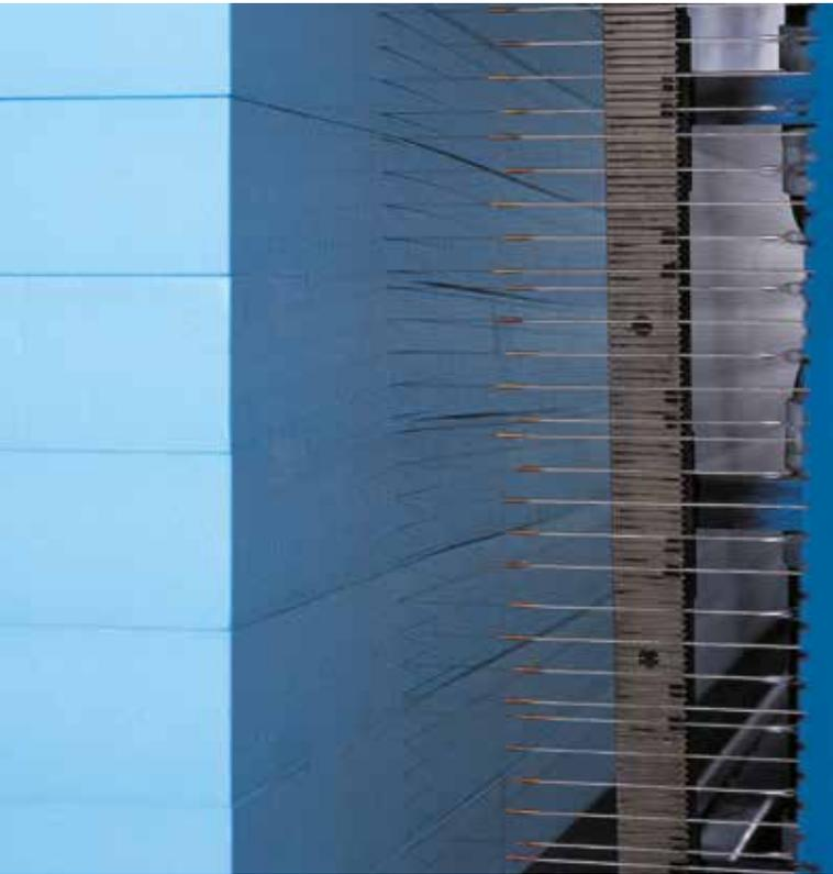
Fig. 08: Oscillating hot wire foam cutting machine for heavy cutting
