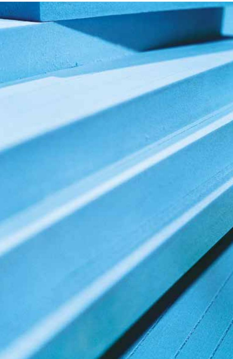
Fig. 02: STYROFOAM™ extruded polystyrene foam
