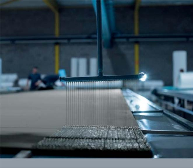
Fig. 16: Application of a 2 component PU adhesive
