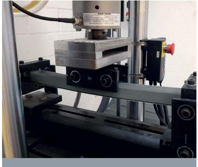
Fig. 13: Dynamic test on sandwich panels with XENERGY™ Ultra core
