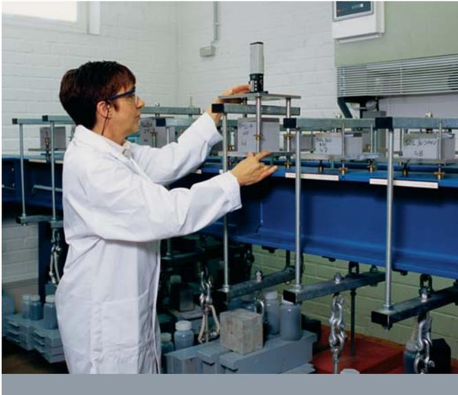
Fig. 11: Testing creep performance in Ravago Building Solutions's dedicated laboratory
