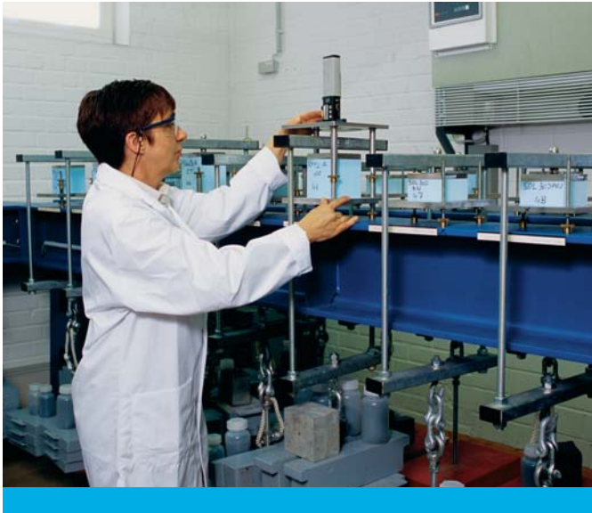
Fig. 10: Testing creep performance in Ravago Building Solutions's dedicated laboratory
