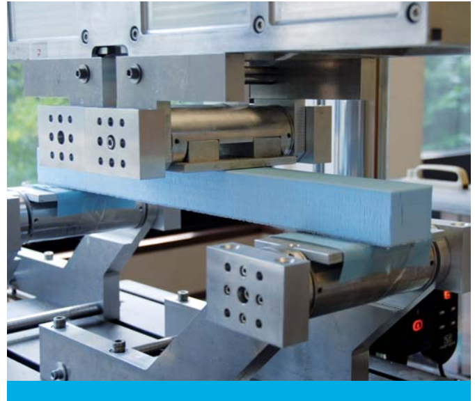
Fig. 12: Dynamic test on sandwich panels with STYROFOAM core
